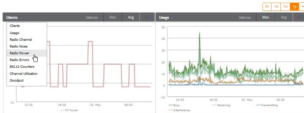
Figure 81: Radio Statistics Interactive Graphs Illustration – Radio Power and Channel Utilization displayed
